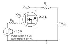
Fig. 10a - Switching Time Test Circuit
