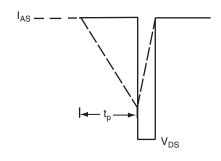
Fig. 12b - Unclamped Inductive Waveforms
