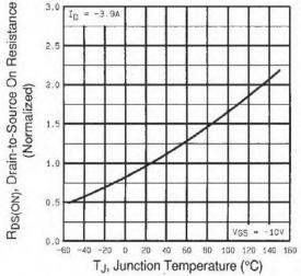
Fig. 4 - Normalized On-Resistance vs. Temperature
