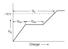
Fig. 13a - Basic Gate Charge Waveform
