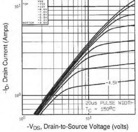
Fig. 2 - Typical Output Characteristics, T<sub>C</sub> = 150 °C
